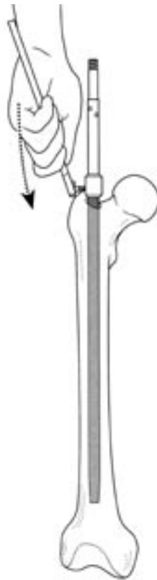
Fig 11. Secure Nail Removal Cap over proximal portion of nail.
