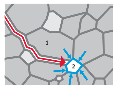
The principle of transformation-toughening by small zirconia particles, which are dispersed in the alumina matrix. 1. Alumina grain; 2. Zirconia grain.
