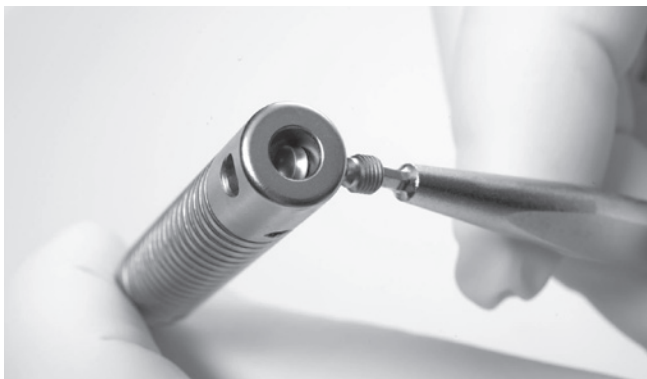
Fig. 6 Loosening the Flex Drill set screw.
